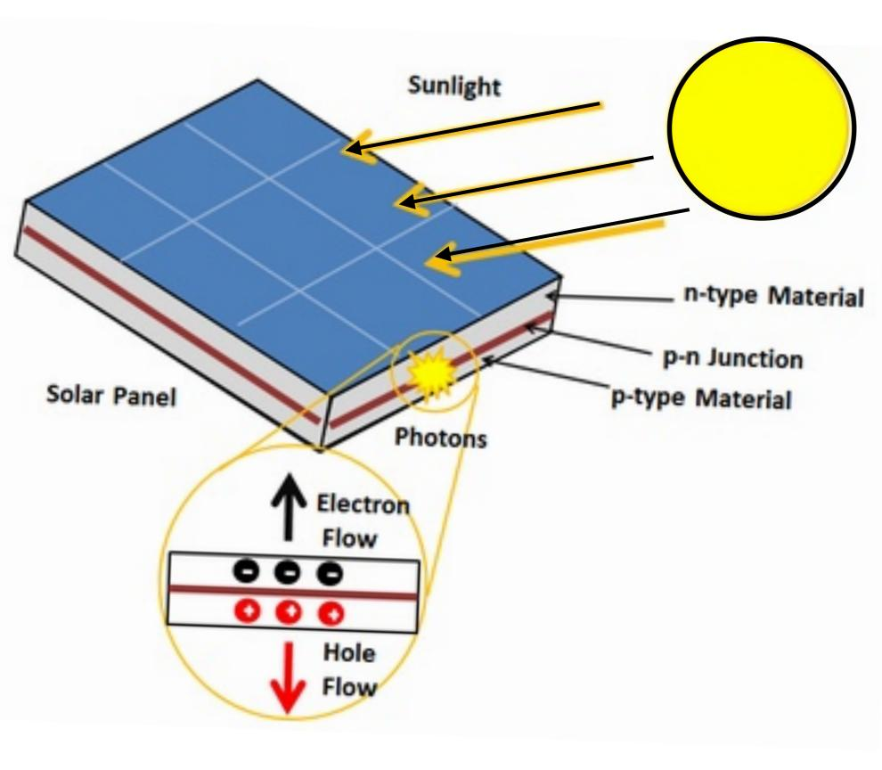
Sunlight causes electrons to flow from negatively charged silicon to positively charged silicon which creates Direct Electrical Current, DC, in a circuit.
