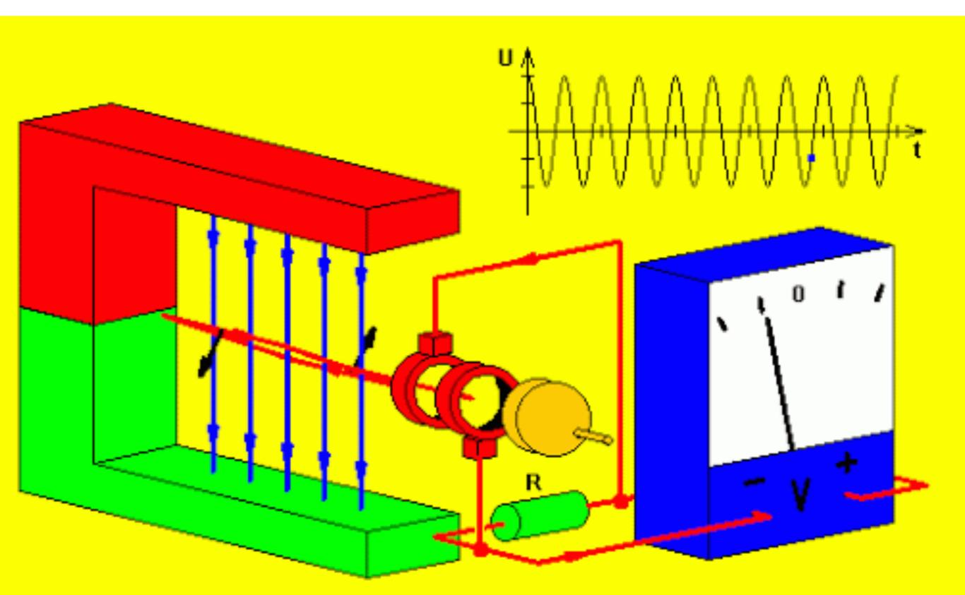
Magnetic field induces electricity into wire
