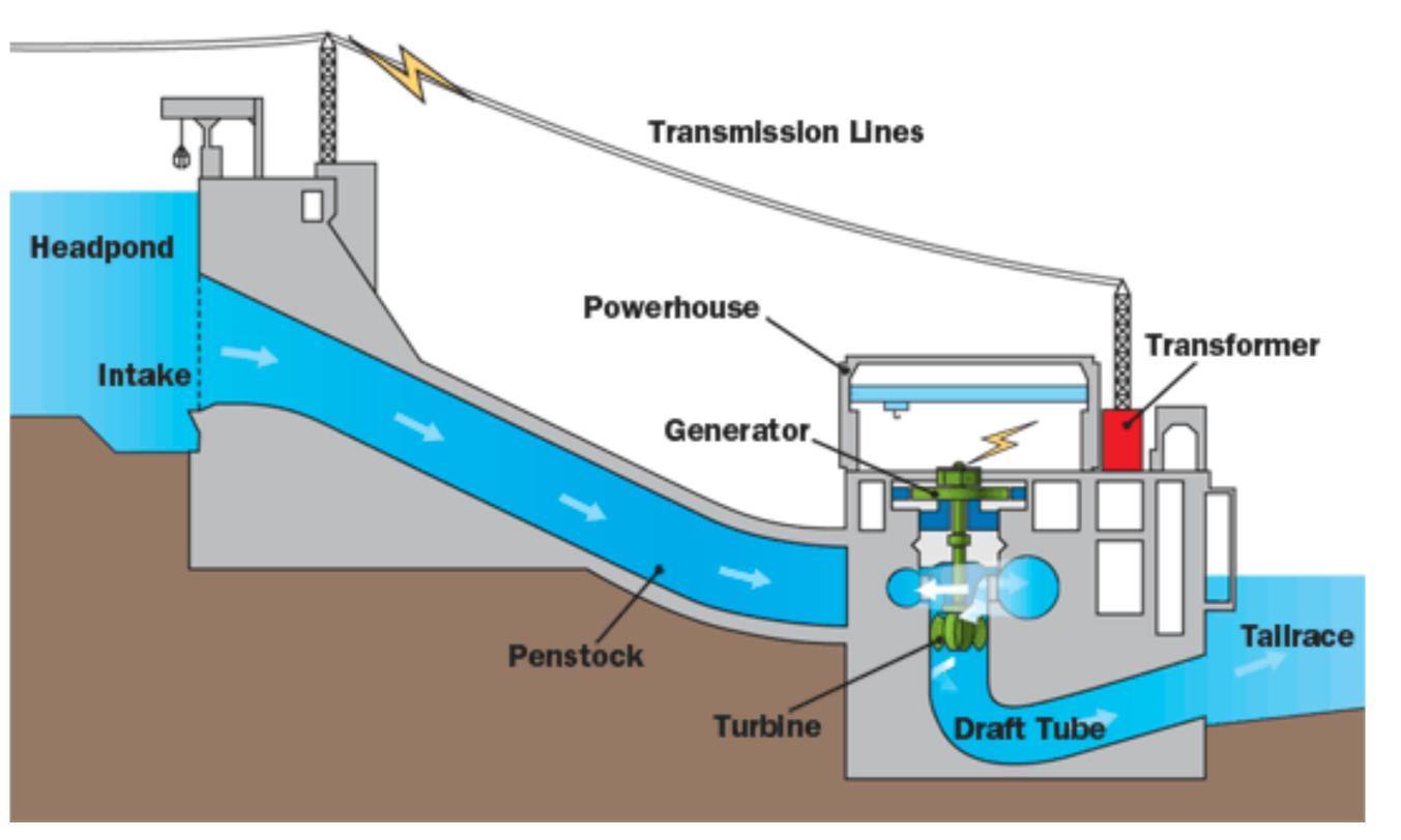
Flowing water pressure turns turbine which turns generator.
